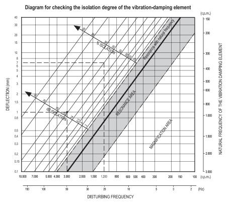
With reference to the graph below the products that intersect the 1400 N line are: AVG, AVM. For the 1400 N load, the expected static deflections are:
